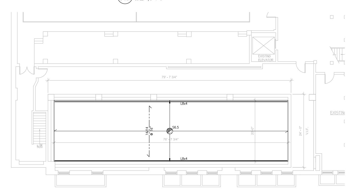
SWIMMING POOL INFIL PLAN-ALTERNATE S-.101 | SCALE: 1/8"=1'-0"
