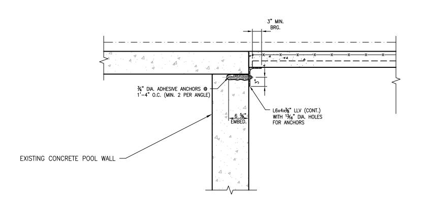
TYPICAL DETAIL SHELF ANGLE AT SIDE WALL FOR COMPOSITE FLOOR DECK SUPPORT SCALE: 1"=1'-0"
